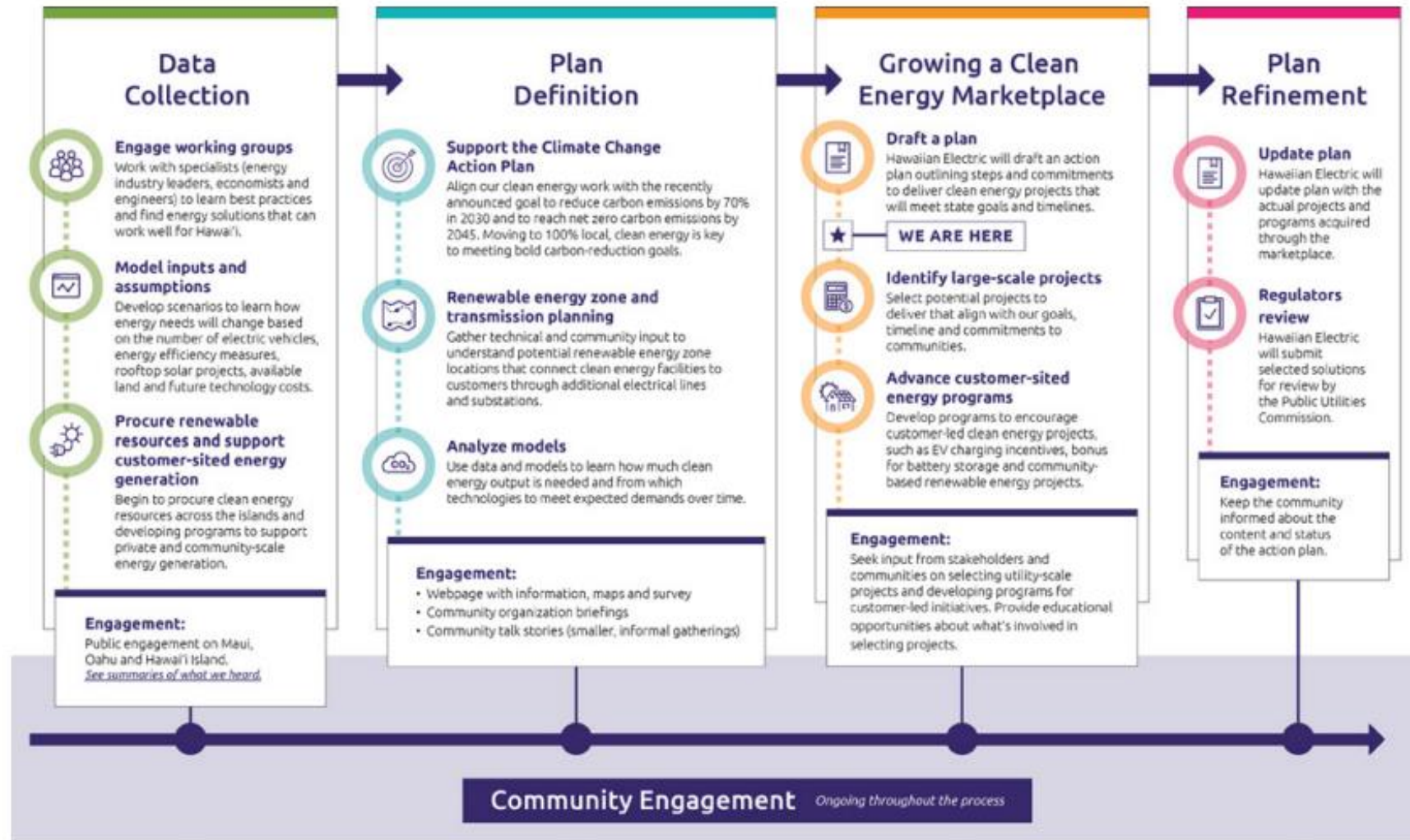
Figure 1-2. High-level steps of Integrated Grid Planning
