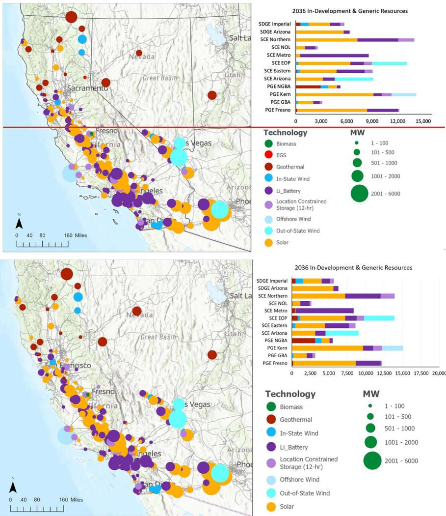
Figure 2: Updated busbar mapping results of the 26-27 TPP base case portfolio 2041 model year. (Left) Map of the final busbar mapping results. (Right) Chart showing mapping results summed by region. Resources shown in MW's.
