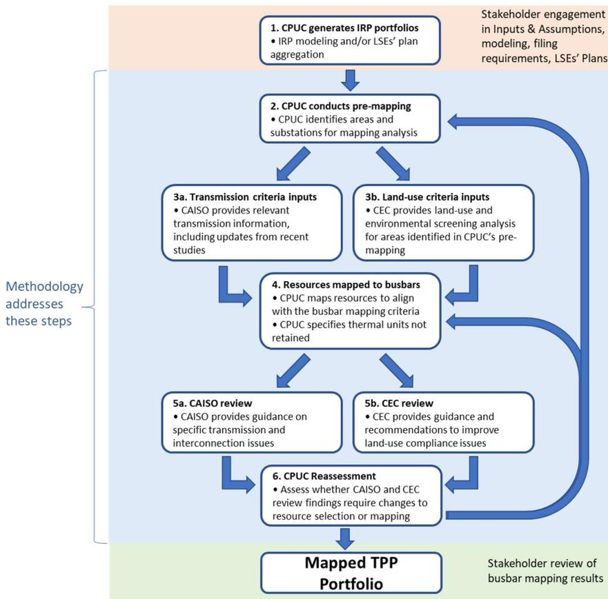
Figure 9 outlines the busbar mapping process, which underwent some revisions prior to the September 2025 Ruling to refine the process and criteria alignment analysis and incorporate new and updated datasets. These changes included:
