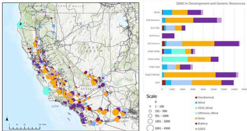
Figure 12: Busbar mapping results of the 26-27 TPP limited wind sensitivity portfolio 2041 model year. (Left) Map of the final busbar mapping results. (Right) Chart showing mapping results summed by region. Resources shown in MWs.
