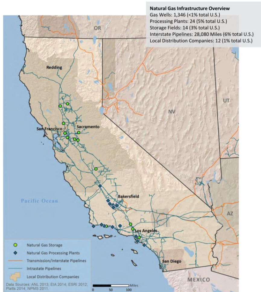
Figure 8. Gas infrastructure in California (reproduced from U.S. DOE 2015). California has 14 gas storage reservoirs in 12 storage fields (EIA 2021).
