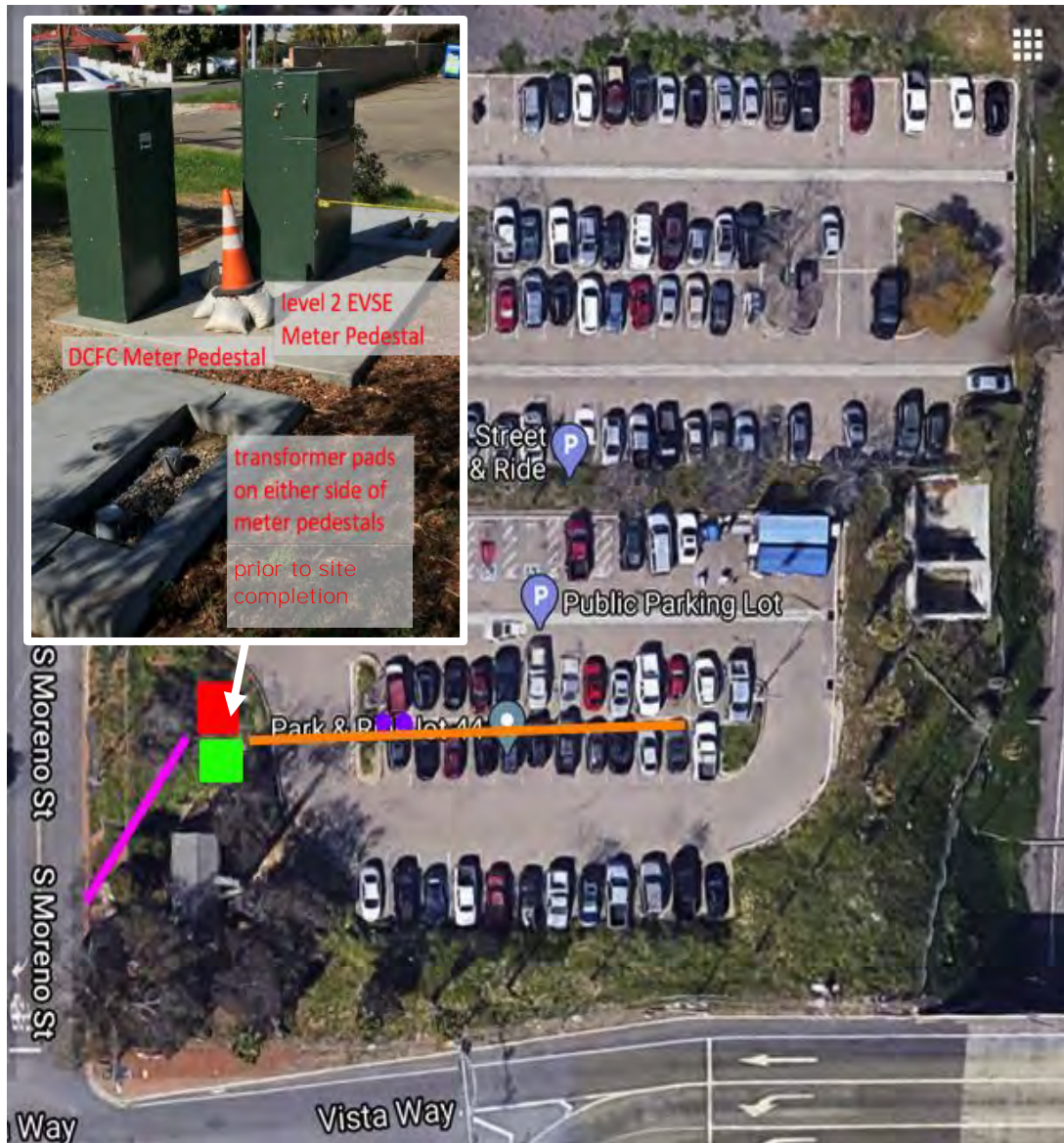
Figure 89. Path of trenching from power source to switchgear and to the chargers
