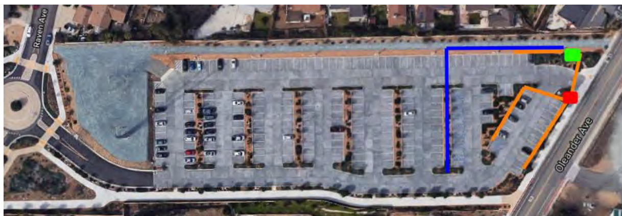
Figure 93. Satellite image of chula vista site with trenching path (orange) and an alternative trenching route to head-to-head parking rows (blue)
