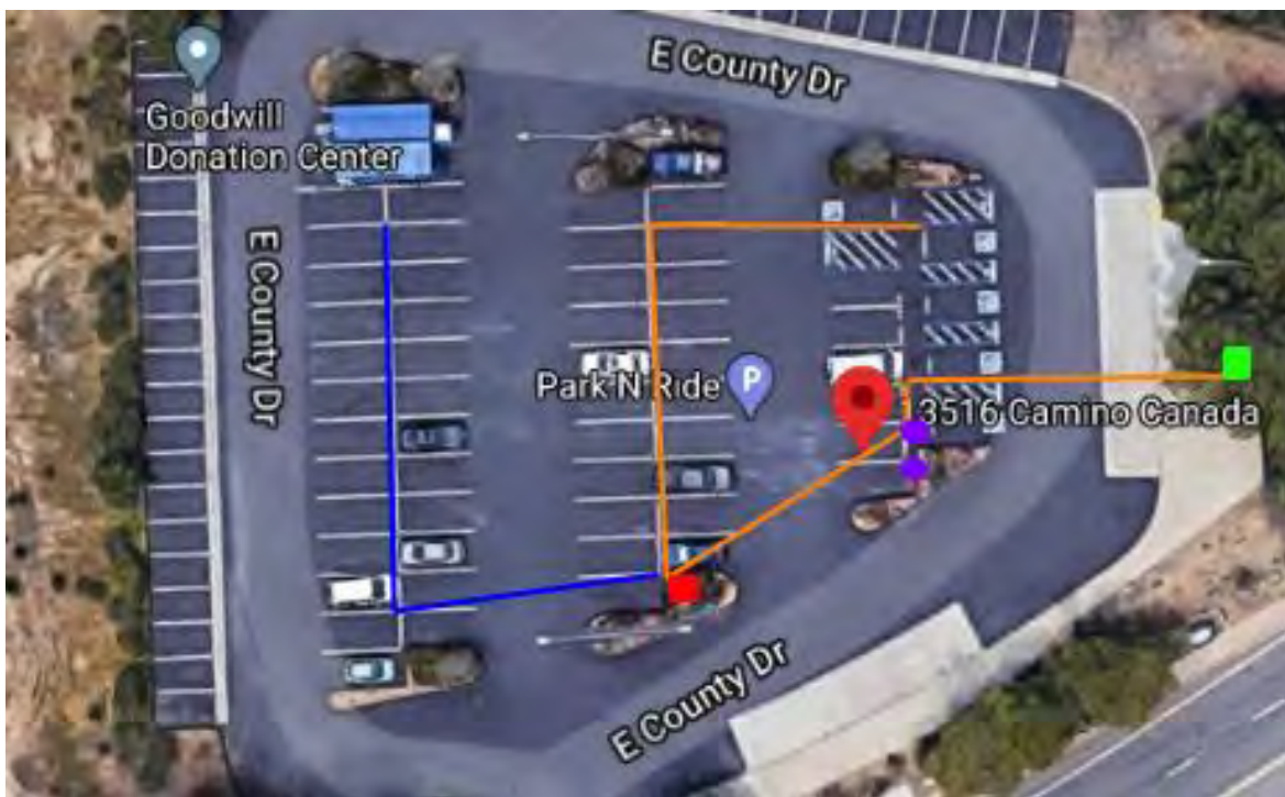
Figure 95. Satellite image of El Cajon site with trenching path (orange) and an alternative trenching route to support greater parking space access to chargers (blue)
