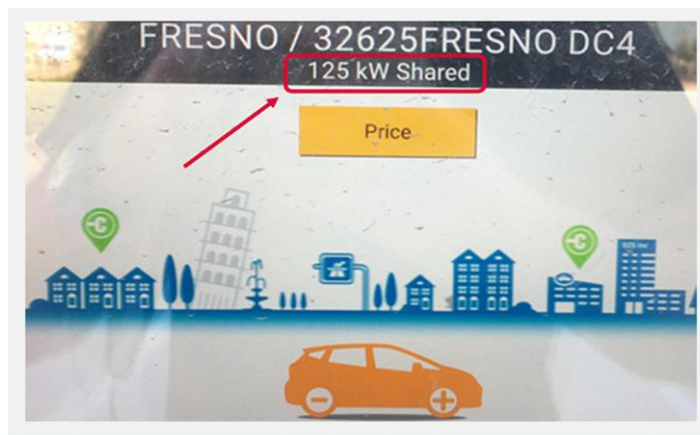
Figure 82. PG&E EV Fast Charge Program Charger Displaying Higher Power Capability than Nameplate
