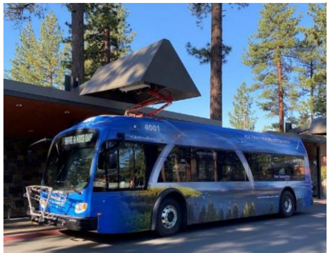
Figure 259. Liberty EV Bus Infrastructure Program TTD’s Proterra Electric Bus Charging at LTCC
