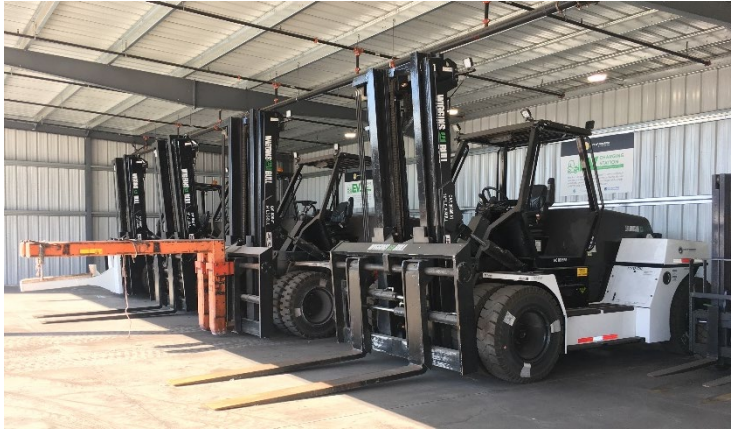
Vehicles illustrative of the site's operational fleet. Left: 36,000-lb-capacity battery-electric forklifts; right: 8,000-lb-capacity battery-electric forklifts
