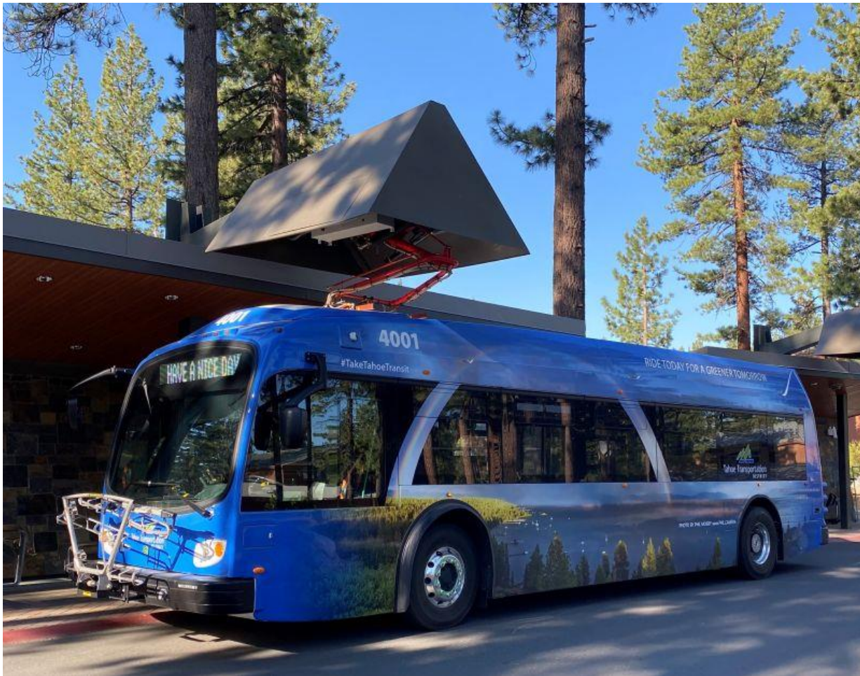
Figure 199. TTD’s Proterra Electric Bus Charging on the 450 kW ABB Pantograph at LTCC
