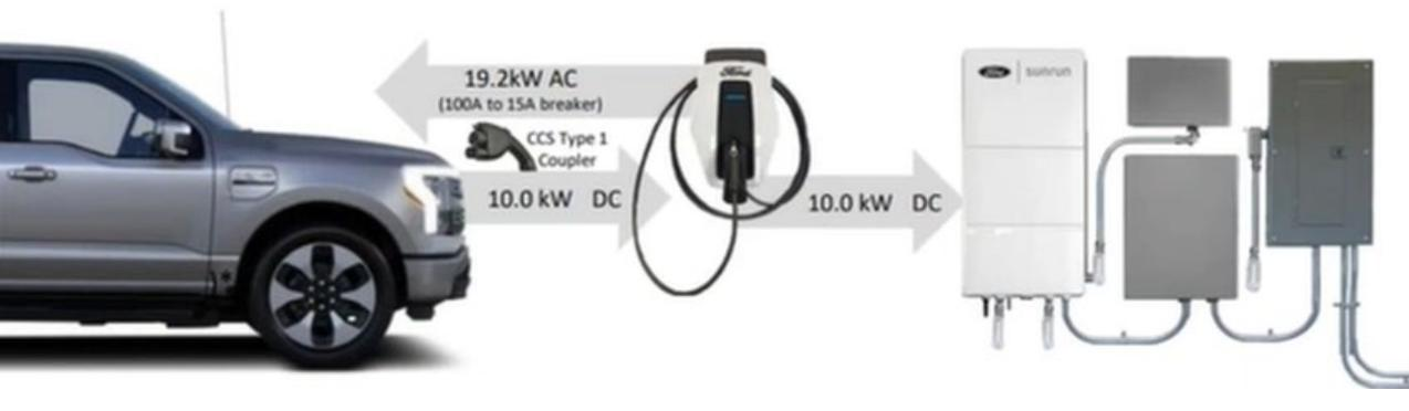
*Most of today's light-duty and medium/heavy-duty equipment capable of bidirectional charging use the DC configuration (i.e., stationary inverter offboard vehicle)*
