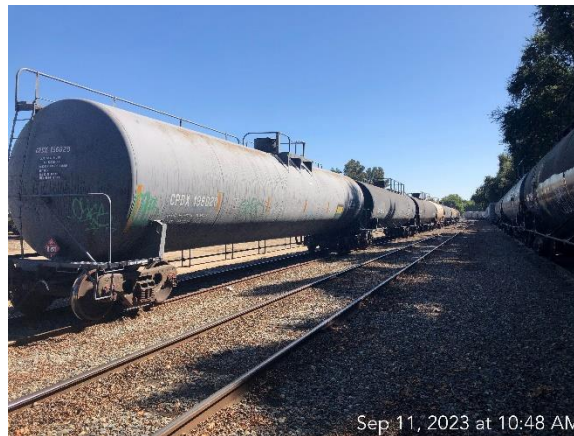
Seven hazardous material tank cars with no handbrakes applied
