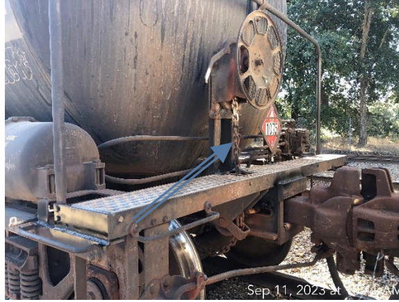
Loose chain indicating handbrake is not applied
