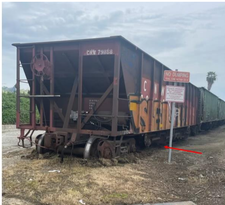
Lead car derailed after rolling off the end of the track
