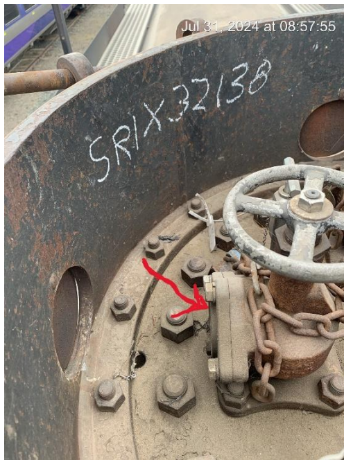
Missing plug on liquid line valve
