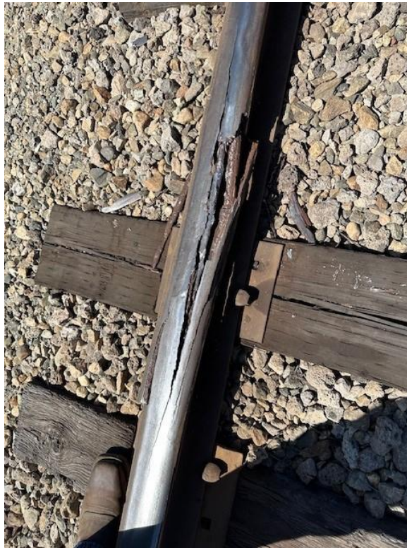
Rail with 48" Vertical Split Head
