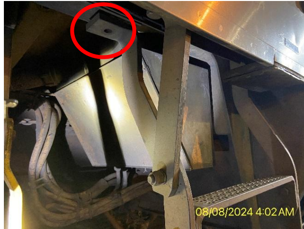
Sill step loose, securement bolt missing.
