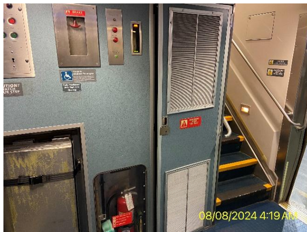
Electrical door panel left open exposing high voltage
