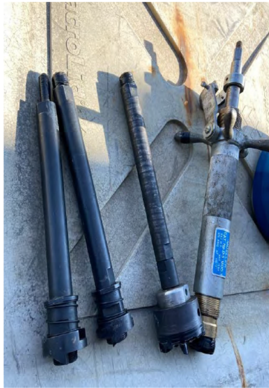
Figure 2. Mueller D-5 machine and inserting tool involved in the incident.
