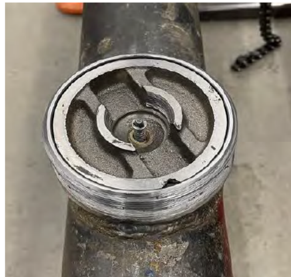
Figure 4. Post Incident Photo- 4” Mueller Line Stopper with damage completion plug but no cap on (top view)
