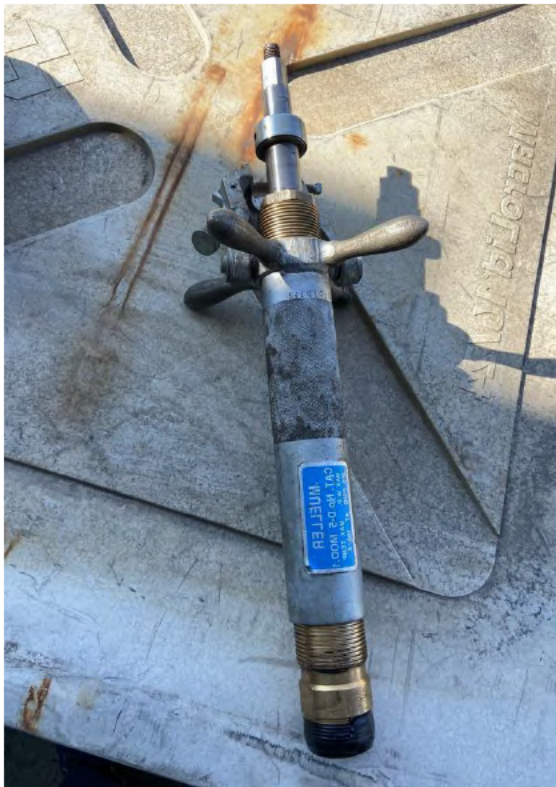
Figure 1. Mueller D-5 machine involved in the incident.
