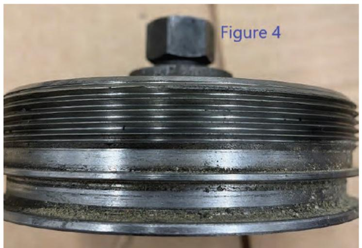
Examination of Mueller H-17190 4" M2 Fitting: Minor damaged noted on leading internal completion plug thread between 12 o'clock and 2 o'clock positions (see Figure 5).
