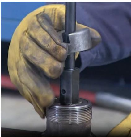
Figure 1: Proper completion plug thread engagement.
