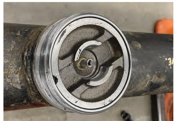
Figure 2: Spring loaded equalization valve on 4" plug.
