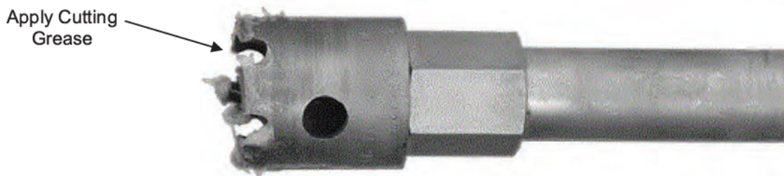
Figure 6. Cutting Grease on Shell Cutter and Pilot Bit
