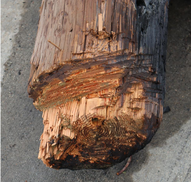
Figure 7: Bottom half of Pole No. 1714303E showing where the pole was most likely cut by the blade-like object.
