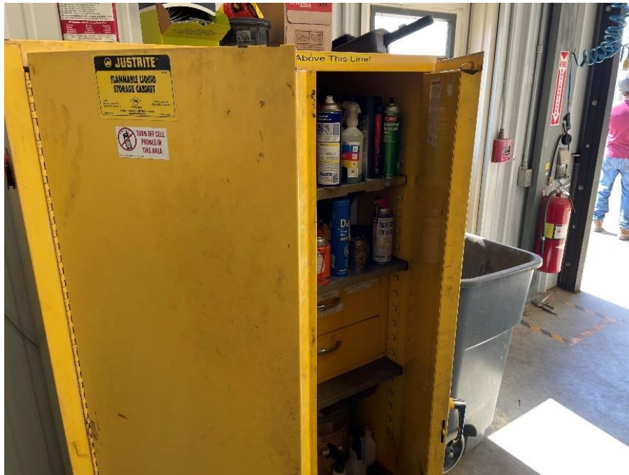
Figure 33: The machine shop flammable material cabinet is missing an NFPA hazard diamond.
