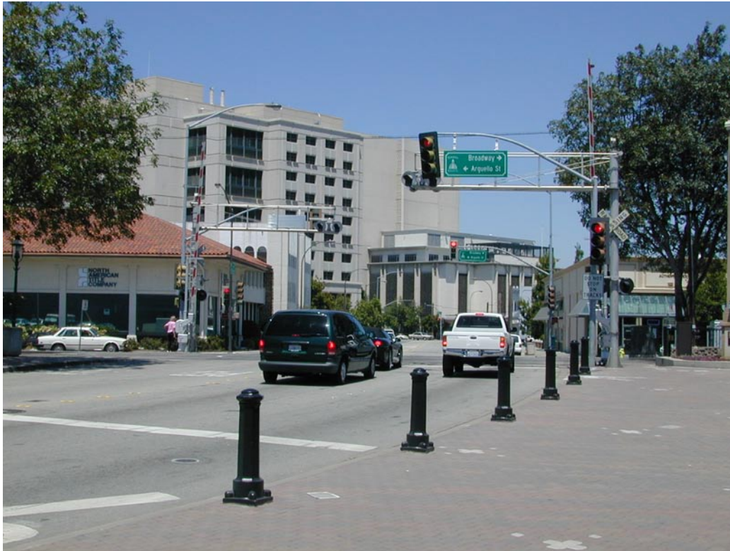
Figure 54. Advance Head, Broadway and Arguello at Caltrain Commuter Line, Redwood City, California
