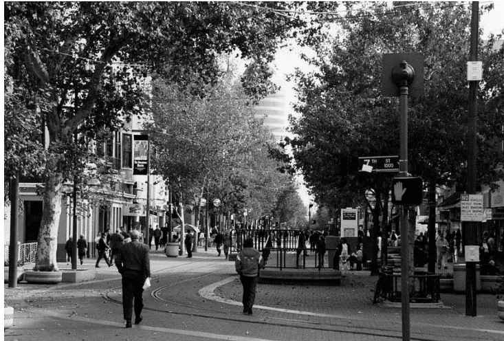
Figure 73. ADA Dynamic Envelope Delineation in Sacramento, California
