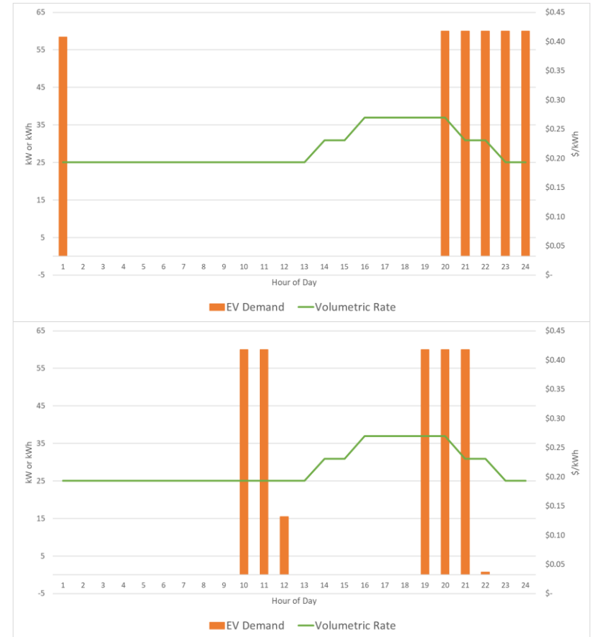
60 kW EVSE, 350 kWh bus battery
