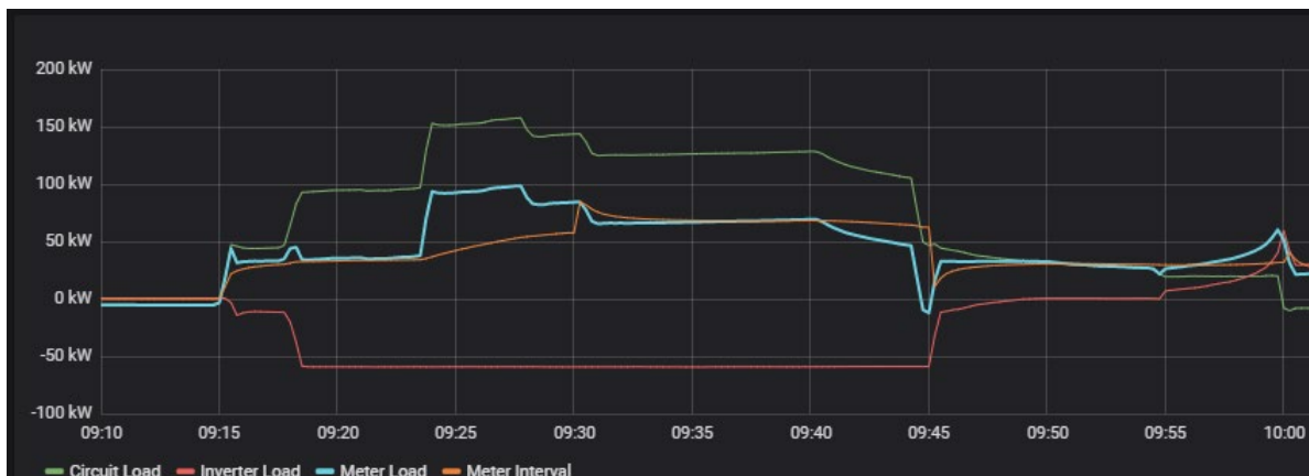
Image 4: Batteries discharging with negative “Inverter Load” value.
