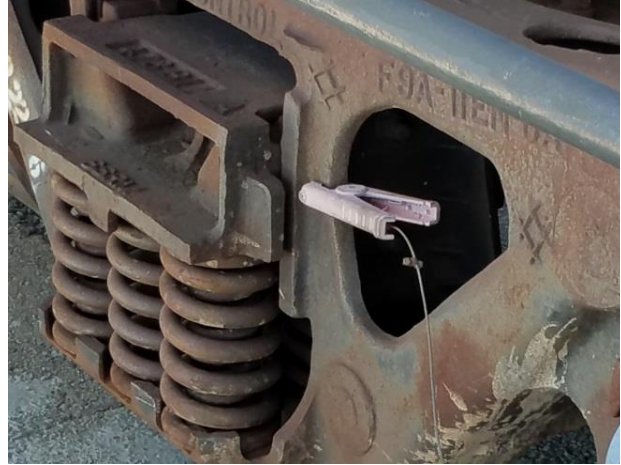
Non-compliant static protection location
