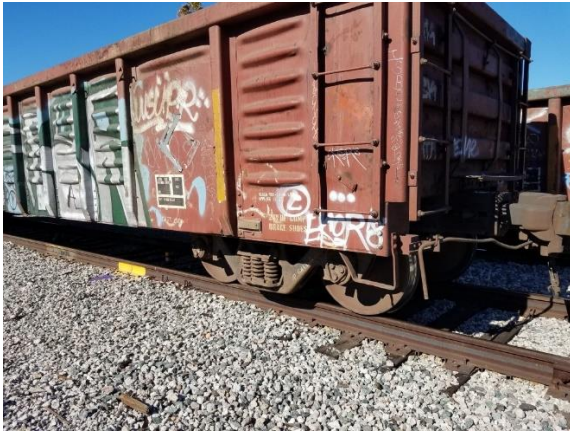
Yellow paint is the designated clearance point; this rail car extends beyond its limit
