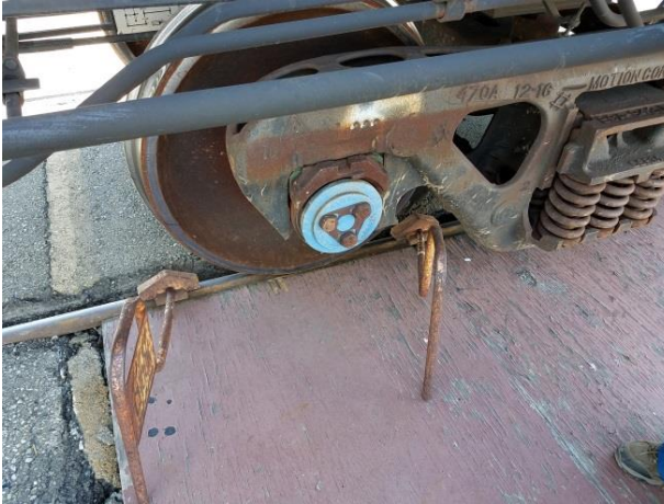
Non-compliant placement of wheel chocks
