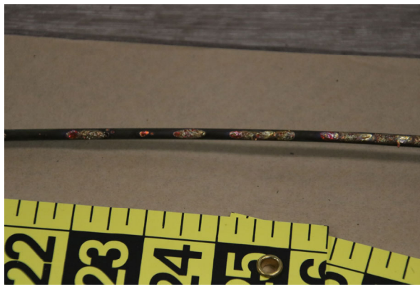
Figure 7: Damaged center conductor.
