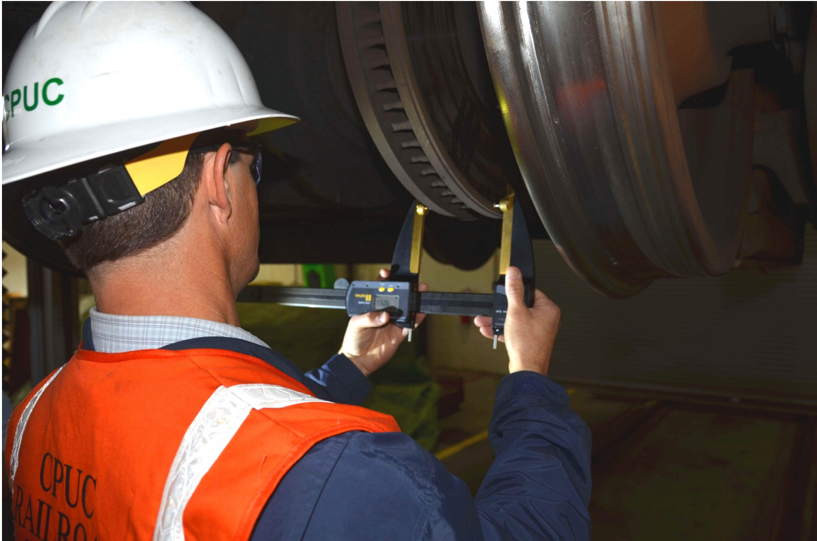
SED inspector measuring powered truck axle rotor wear
